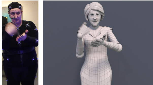
Figure 2: Motion capture session: the real signer from the recorded video (left) and the 3D mesh of the corresponding virtual signer (right)
